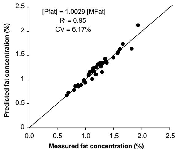
**Figure 4.** Fit of whey fat concentration and sidescatter ratio  $S_{875/425}$  to equation 1. [PFat] is predicted fat; [MFat] is measured fat;  $N = 34$ ; and  $R^2$  and CV values corresponded to the fit of the three experimental batches.
