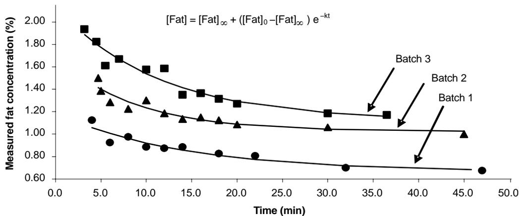
Figure 2. Plot of measured whey fat concentration as a function of time. Solid lines represent least squares fit of a first order kinetic equation (eq. 2) to the measured whey fat concentration. Data obtained during three different manufacturing processes of “Ripened Murcia Cheese.” Whey fat concentration determined by Gerber method.
