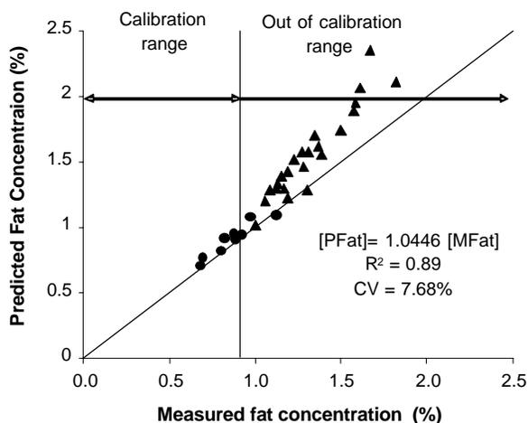
**Figure 3.** Prediction of whey fat concentration using the sidescatter ratio  $S_{875/425}$  and equation 1. [PFat] is predicted fat; [MFat] is measured fat (Gerber method);  $N = 34$ ; and  $R^2$  and CV values corresponded exclusively to the prediction of fat concentration for batch number one (●). Data points for batches two and three (▲).
