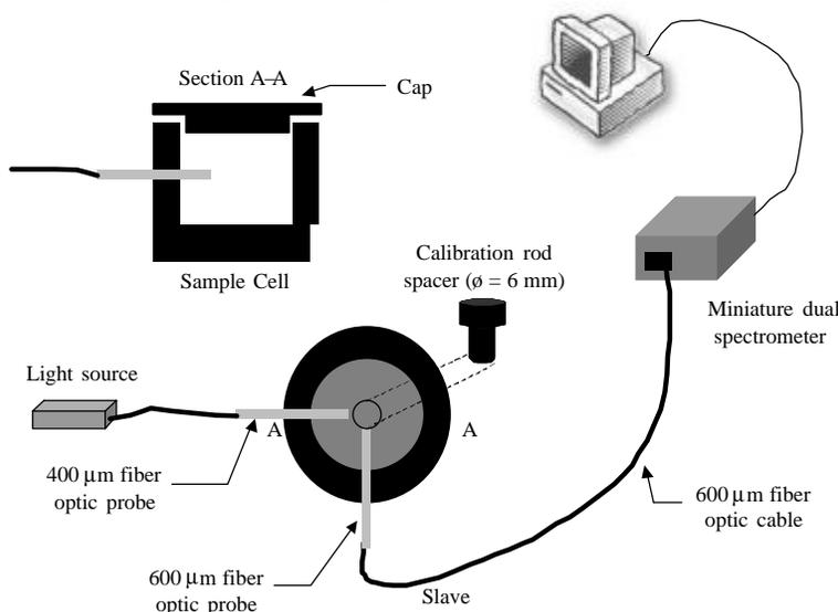
Figure 1. Schematic of optical configuration used to determine whey fat concentration in whey using light sidescatter at 90°.
