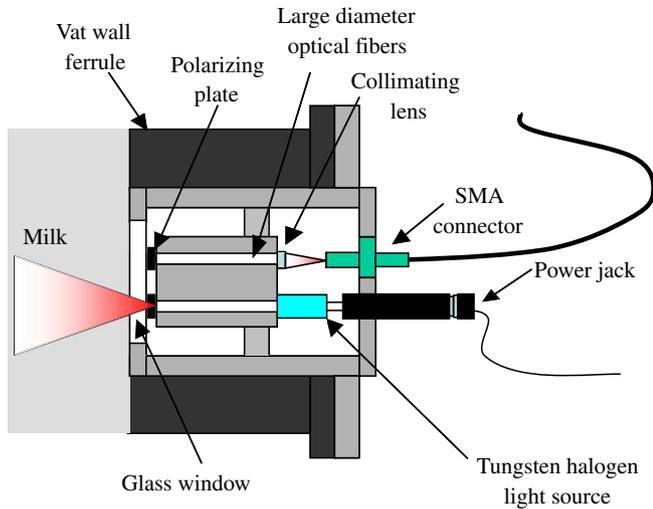
**Fig. 1.** Schematic of the novel large field of view (LFV) colour sensor and optical configuration employed for monitoring curd syneresis.
