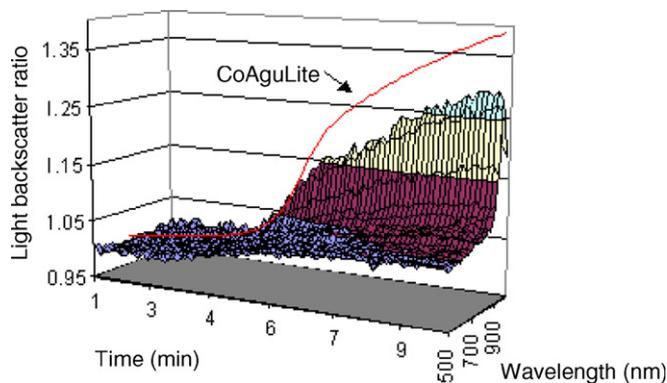
Fig. 3. Typical large field view (LFV) sensor response during coagulation (temperature = 38.4 °C;  $\text{CaCl}_2 = 156 \text{ mg kg}^{-1}$ ) at wavelengths between 500 and 1000 nm and the simultaneous CoAguLite™ response.
