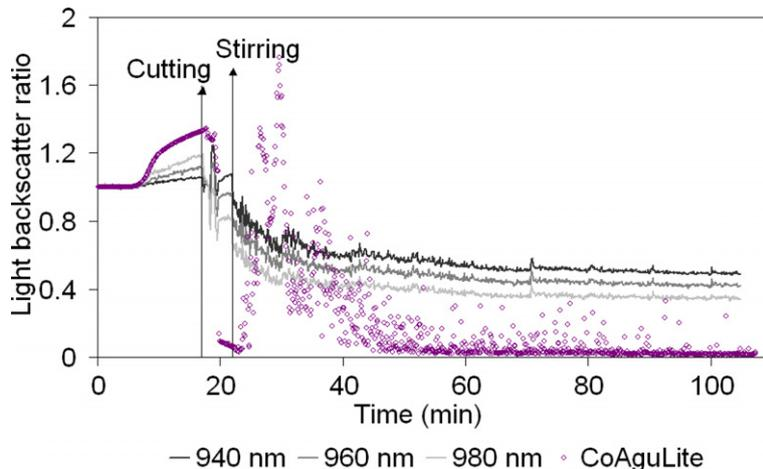
Fig. 4. Typical sensor profiles of the large field view (LFV) sensor at 940, 960 and 980 nm and the CoAguLite™ sensor during coagulation and syneresis (temperature = 30 °C;  $\text{CaCl}_2 = 156 \text{ mg kg}^{-1}$ ).
