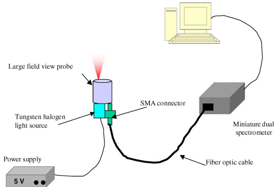
Fig. 1. Schematic of the large field view sensor configuration.
