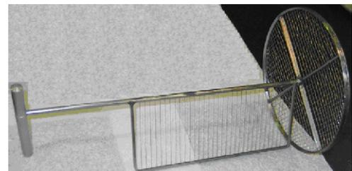
Fig. 2. The coagulum cutting knife.
