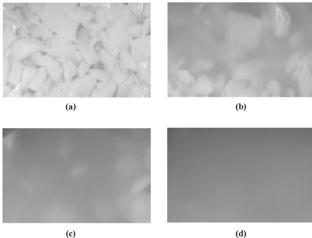
**Figure 2.** Computer vision images of the curd/whey mixture at a) 5 min, b) 15 min, c) 35 min, and d) 85 min after cutting, in the 10-L vat. The curd/whey mixture is being stirred by twin stirrers (Figure 1).
