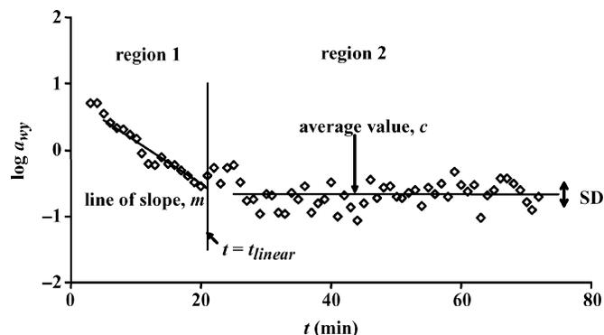
**Figure 5.** Graph of  $\log a_{wy}$  (log of ratio between white and yellow areas) vs. time after cutting the coagulum for a typical trial, using the computer vision system. It is apparent that  $\log a_{wy}$  decreases in a linear manner up to  $t_{linear}$ , the vertical bar indicating the point of departure from this first linear section.
