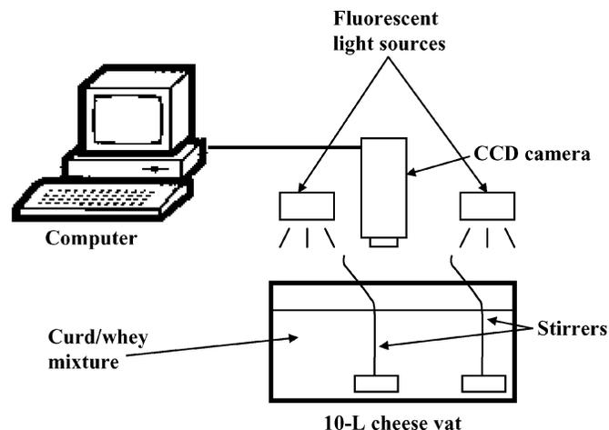
**Figure 1.** Schematic of computer vision system coupled to the cheese vat with twin corotating stirrers. CCD = charge-coupled device.
