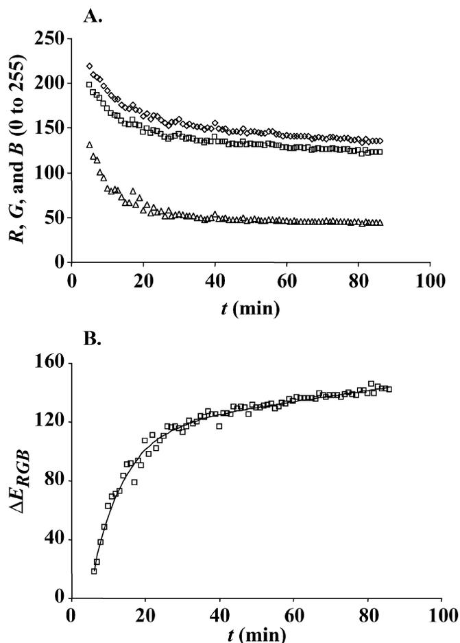
**Figure 3.** a) Red ( $\diamond$ ), green ( $\square$ ), and blue ( $\triangle$ ) (i.e.,  $RGB$ , values on a scale of 0 – 255 for a trial) and b) the corresponding  $\Delta E_m$  values (—;  $RGB$  model) fitted to  $\Delta E_{RGB}$  values ( $\square$ ) vs. time.  $\Delta E_m = \Delta E_0 [1 - e^{-k_1(t-t_0)}] + k_2 t$ .  $\Delta E_{RGB} = \sqrt{(\Delta R)^2 + (\Delta G)^2 + (\Delta B)^2}$ .
