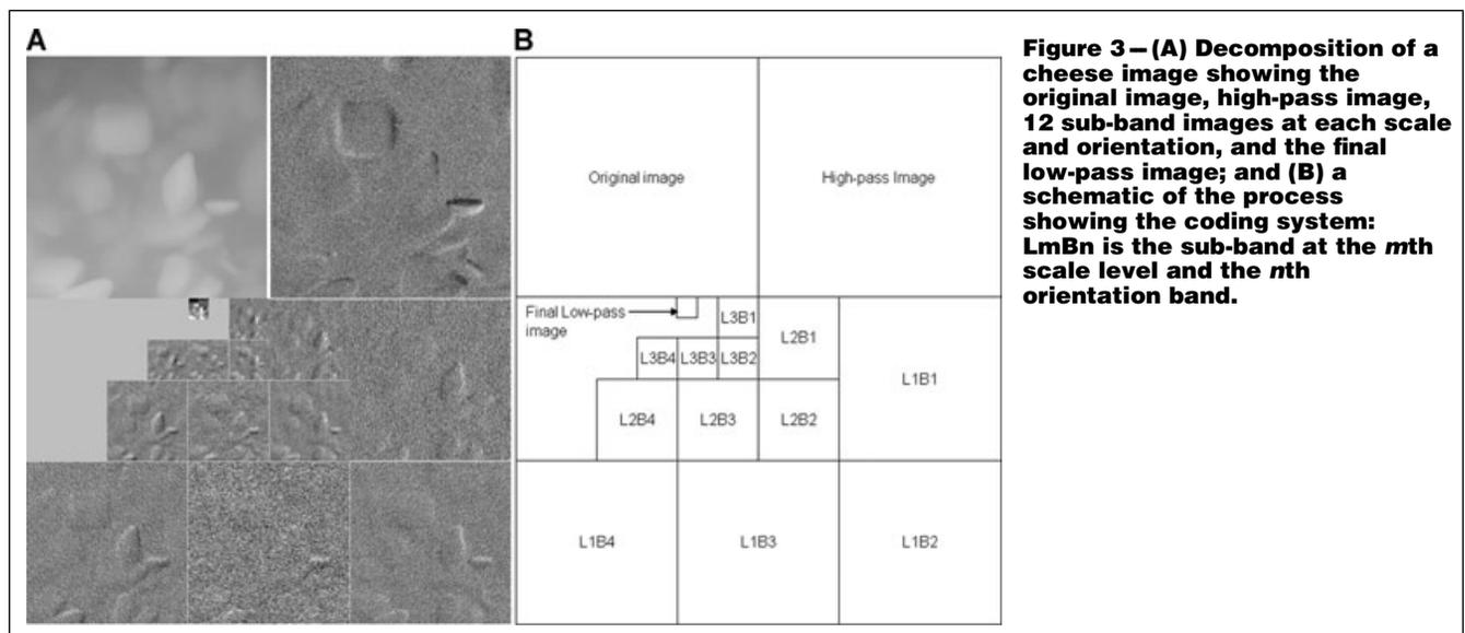
**Figure 3 – (A) Decomposition of a cheese image showing the original image, high-pass image, 12 sub-band images at each scale and orientation, and the final low-pass image; and (B) a schematic of the process showing the coding system:  $LmBn$  is the sub-band at the  $m$ th scale level and the  $n$ th orientation band.**
