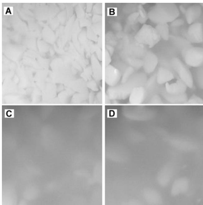
**Figure 2—A sequence of images captured during the syneresis process at (A) 4, (B) 14, (C) 24, (D) 34 min after gel cutting time.**
