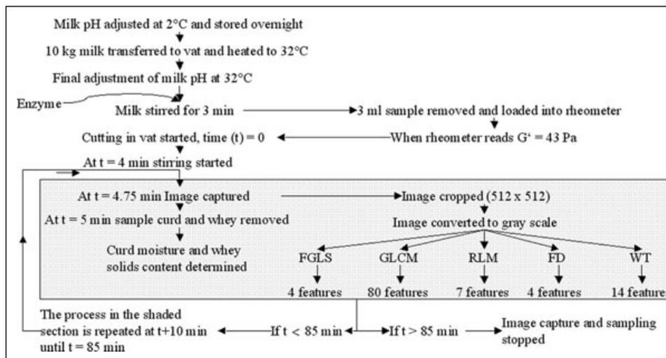
**Figure 1** – Flow diagram of the procedures employed for experimental trials and analysis, and extracting image texture features.
